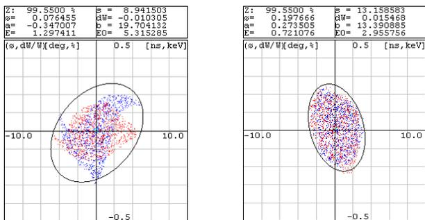
Figure 1: Longitudinal phase spaces at the output of RIA segment1 for  $U^{28+,29+}$  beam with old cavity tuning procedure (left) and new tuning procedure using the algorithm (right). The multi-q effective emittance is plotted around all charge states.
