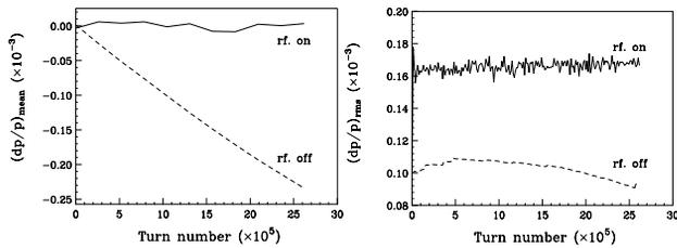
Figure 2: Simulation results showing the mean value (left) and rms value (right) of the relative momentum difference vs the turn number for both rf on and rf off.
