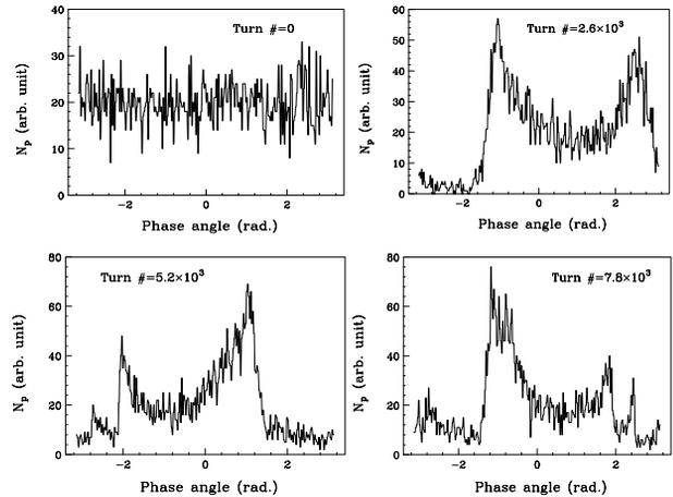
Figure 3: Simulation results showing the synchrotron oscillation of two bunches in the stationary bucket, which occurs when the rf comes on after the target interaction has been ongoing for  $3.66 \times 10^6$  turns.
