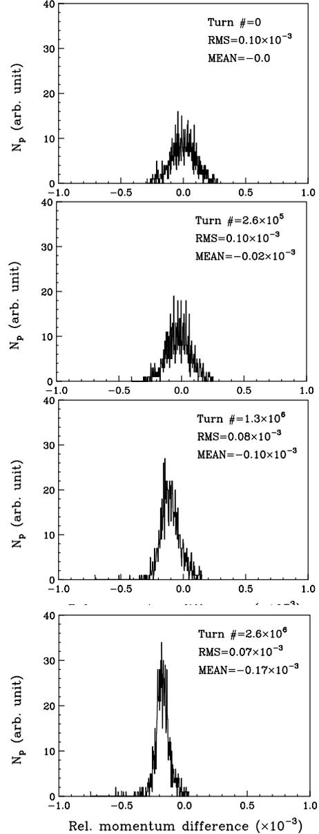
Figure 1: Simulation result showing the history of particles' distribution in the momentum space. The turn number, the rms and mean values of the relative momentum difference are indicated. The target stream is assumed to be within (-1,+3)mm of the central orbit.
