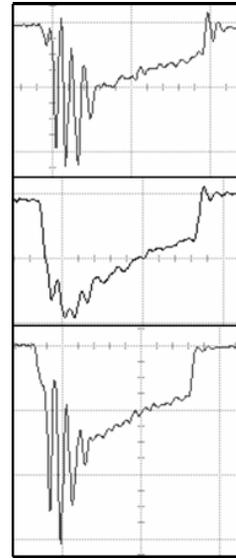
Figure 2: Beam current measured at 0.83 m (top), 3.23 m (middle), and 5.78 m (bottom) downstream from the cathode.
