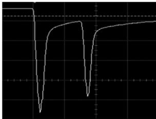
Figure 4: Sample optical pulse train. Up to four pulses could be produced.
