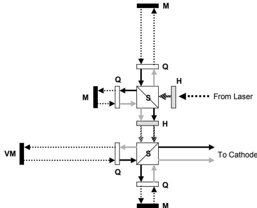
Figure 3: Optical modulation system, showing polarized beam splitters (S), half wave plates (H), quarter wave plates (Q), fixed-distance mirrors (M) and variable-distance mirror (VM). Arrow colors and styles correspond to light polarization states.
