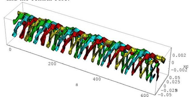
Figure 3: 3D view of the beamlets along the circumference of the PS ring. Although this is a single structure four-turn long, four colours have been used to ease the visualisation. The fifth beamlet, corresponding to the central core, is not shown here.
