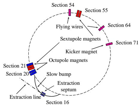
Figure 4: Schematic layout of the PS ring with the elements used for the experimental study of the novel multi-turn extraction.
