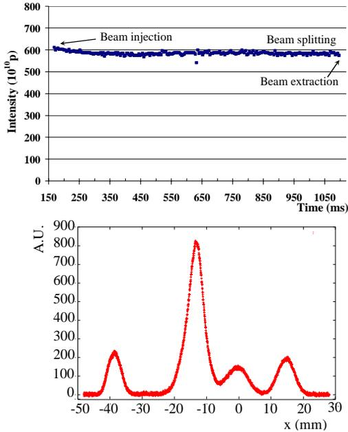
Figure 5: Best result achieved with a high-intensity beam, whose intensity as a function of time (upper) and horizontal beam profile at the end of the capture process (lower) is shown. The profile is not centred at zero due to an instrumental offset of the wire position.
