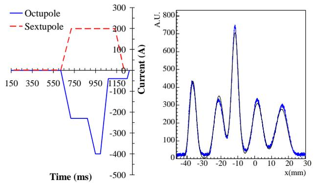
Figure 6: Typical time-dependence of the sextupole and octupole strengths used in the experiment (left). The horizontal beam profile after splitting is shown for the case of the largest fraction of trapped particles (right). The profile is not centred at zero due to an instrumental offset of the wire position.
