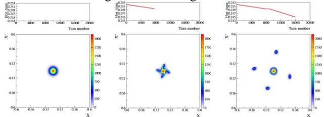
Figure 2: Evolution of the beam distribution during resonance crossing: the initial state is represented by a bi-Gaussian beam (left), at resonance-crossing some particles are trapped inside the moving islands (centre), at the end of the process, the particles trapped in the islands are moved towards higher amplitudes (right).
