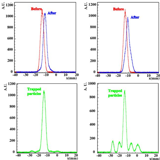
Figure 8: Dependence of the beamlets parameters on the resonance crossing speed. The horizontal profiles for a fast crossing (5 ms) are shown in the left part, corresponding to the three moments, while the profiles on the right correspond to a slower crossing (90 ms). The profiles are not centred at zero due to an instrumental offset of the wire position.
