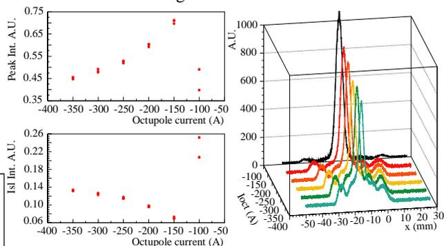
Figure 9: Influence of the octupolar strength on the fraction of particles trapped in the beamlets (upper left) with respect to the intensity in the central core (lower left). The corresponding horizontal beam profiles are also shown (right part).
