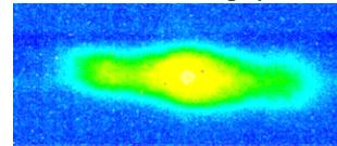
Figure 7: Two-dimensional beam distribution in physical space of the split beam in the transfer line downstream of the PS extraction point.
