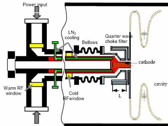
Figure 6: Schematic view of the axial RF power input into the gun half-cell of a superconducting cavity.
