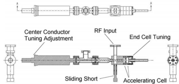
Figure 1: Schematic view of the two cell X-band gun.
