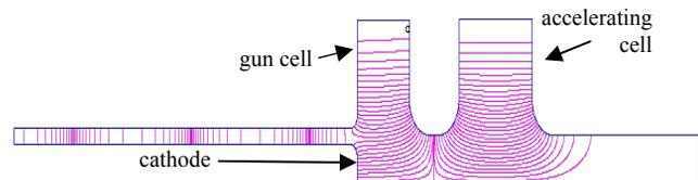
Figure 2: Field distribution in the cavity and coupler.
