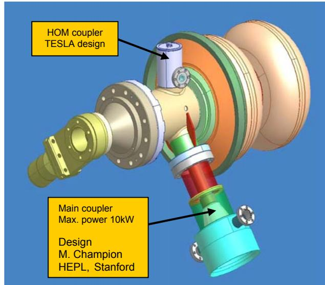
Figure 5: RF power coupler of the ELBE accelerator.
