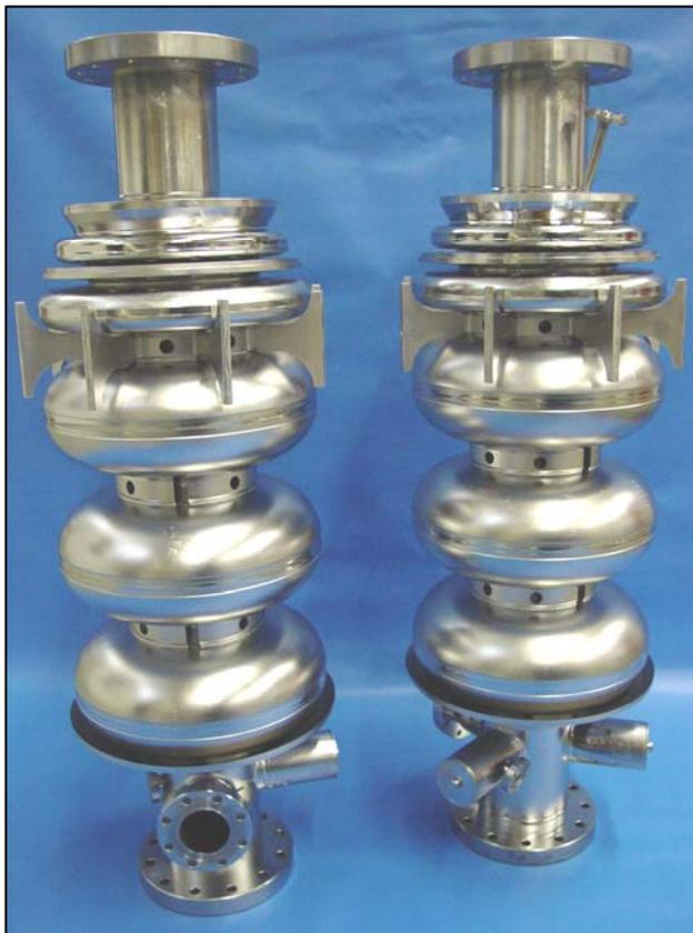
Figure 4: 3½ cell FZR SRF cavity.
