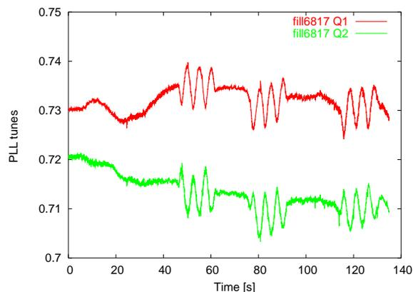
Figure 1: The tunes from the coupling angle modulation.
