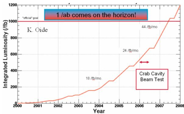
Figure 15. KEKB projected integrated luminosity to 2008.
