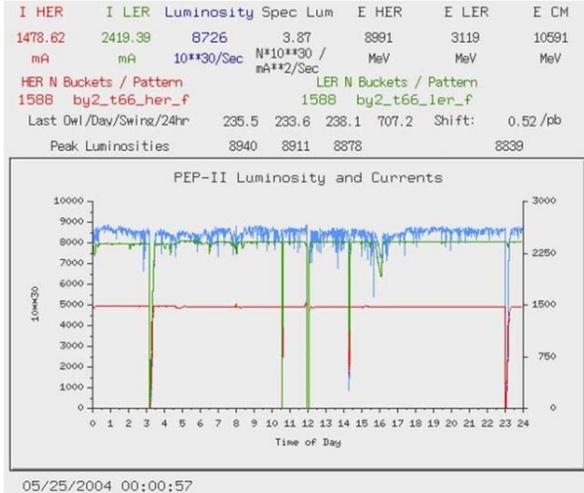
Figure 10 PEP-II trickle charge operation with constant currents and luminosity.
