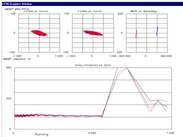
Fig.1 RIAPMTQ simulation results for two charge states (28 in black and 29 in red) of uranium 238. Two matched initial random input beam distributions were generated at the entrance of the RFQ. Bottom plots show rms x and y values for the two beams. The two beams were tracked simultaneously through the RFQ and MEBT. The MEBT begins at 4 meters.
