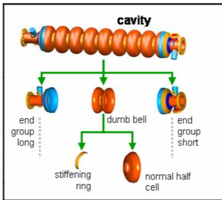
Figure 2: Design view (part breakdown structure).
