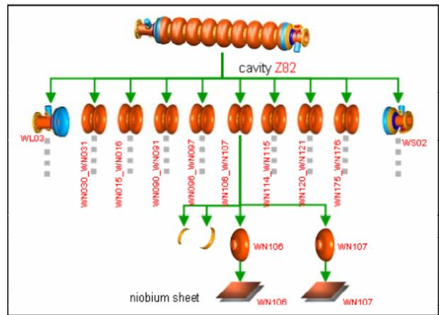
Figure 3: Serialized parts with serial numbers (manufacturing view).
