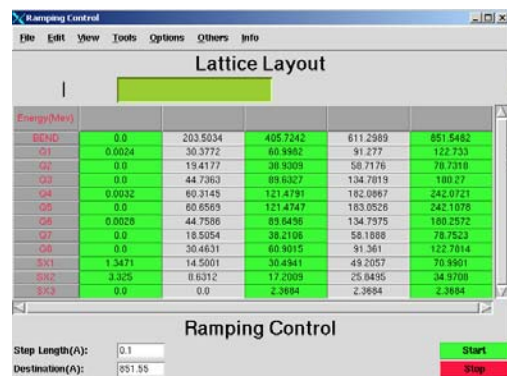
Figure 2: The panel of HLS beam ramping control.
