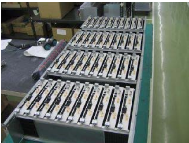
Figure 3: The timing control transmitter (right) and receiver (left) modules.
