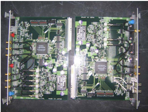
Figure 3: The timing control transmitter (right) and receiver (left) modules.
