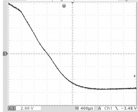
Figure 2: Output signal of the phase detector for booster master oscillator. The phase lock loop is closed at the moment, when signal is crossing zero voltage, while traveling to negative. Scaling of the output is 4V/ns.
