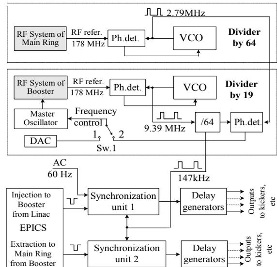
Figure 1: Block-diagram of the timing system.
