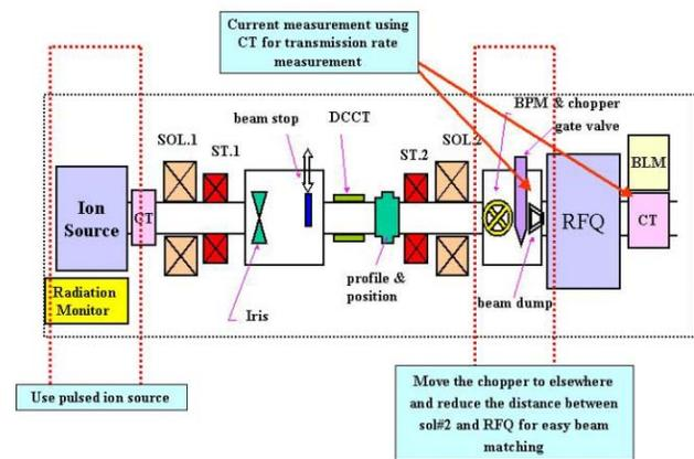
Figure 1: Structure of PEFP RFQ & DTL Devices [5].
