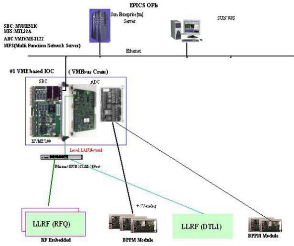
Figure 2: Structure of Upgrade RF Control System.
