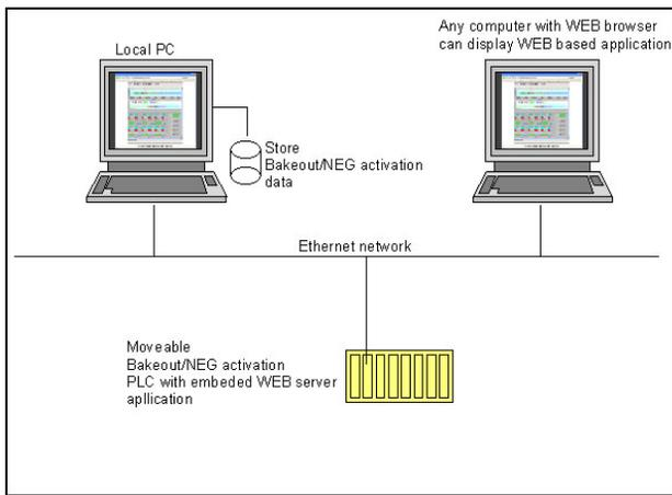
Figure 4: Monitoring and archiving of bake out data.
