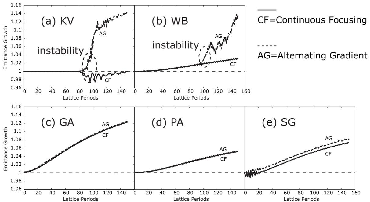
Figure 2: Evolution of the rms emittance during the final beam bunching, (a) for KV, (b) for WB, (c) for GA, (d) for PA, and (e) for SG beams, respectively. Solid curve shows the emittance growth for CF lattice, and the dashed line indicates one with AG focusing lattice.
