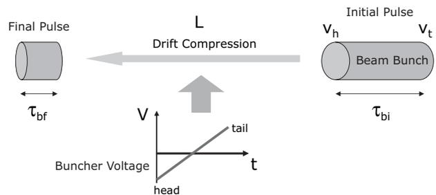
Figure 1: Drift bunch compression by bunching voltage applied at beam buncher at the final stage of HIF driver system.
