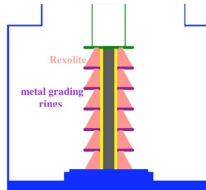
Figure 2: Anode stalk support insulator.
