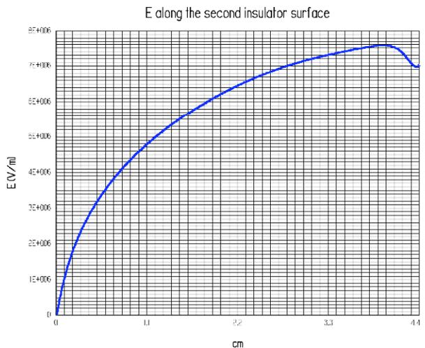
Figure 7: E along the second insulator surface. Electric field varies from 0 to 80 KV/cm on the vertical axis.
