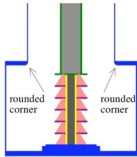
Figure 8: Configuration with the rounded corner in the junction of two MITL chambers.
