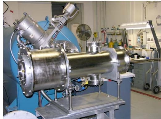
Figure 11: Insulator (inside the chamber) and the anode stalk protruding from the vacuum chamber to the right (MITL removed).
