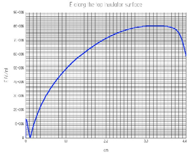
Figure 6: E along the top insulator surface. Electric field varies from 0 to 90 KV/cm on the vertical axis.
