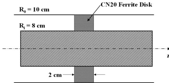
Figure 5: Coaxial transmission line with ferrite insert.
