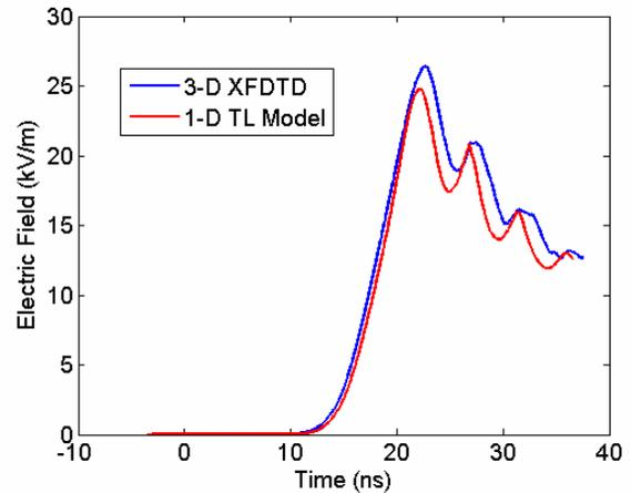
Figure 7: Electric field 1.1 cm after ferrite insert.
