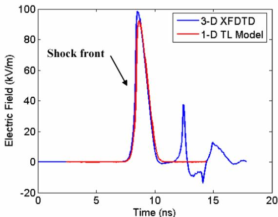
Figure 4: Electric field 25 cm after dielectric insert.
