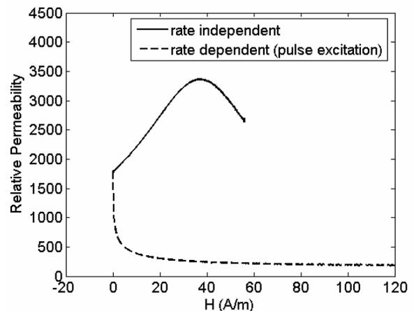
Figure 8: CN20 permeability from XFDTD code.
