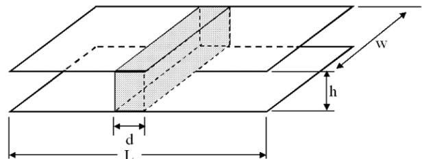
Figure 1: Stripline with block of nonlinear dielectric.
