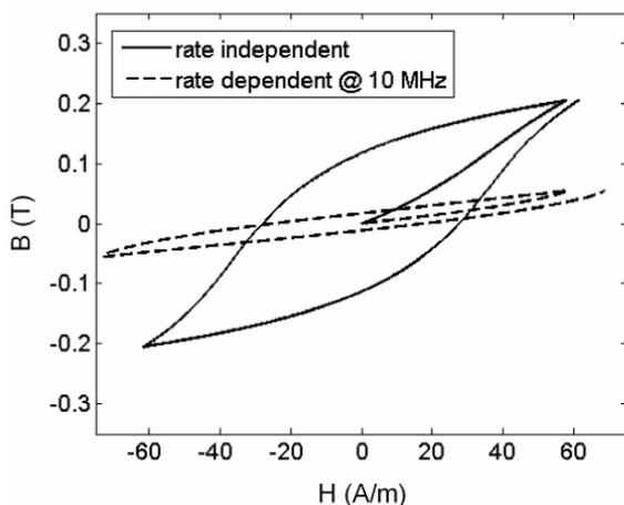
Figure 6: Hysteresis curves for CN20 ferrite.
