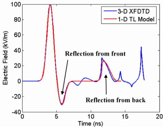
Figure 3: Electric field 25 cm before dielectric insert.
