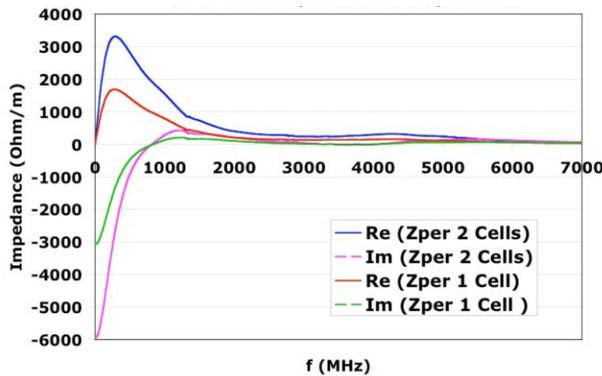
Figure 4: Wakefield impedance for a 5-inch DWA stack cell and for two 5-inch cells separated by 2 inches.
