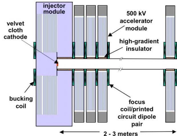
Figure 1: Dielectric wall induction accelerator configuration.
