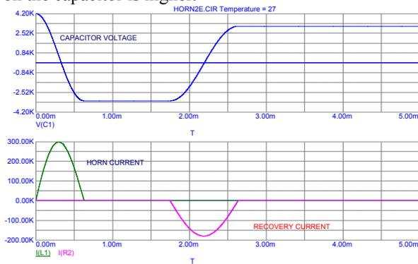
Figure 4: Horn system with recovery circuit: Capacitor voltage, horn current, and recovery current waveform simulations.
