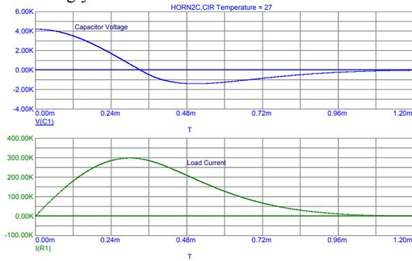
Figure 3: Capacitor voltage and horn current waveform simulations.
