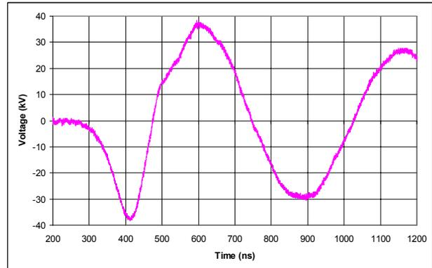
Figure 6: Initial high voltage waveform on the oil dielectric helix.
