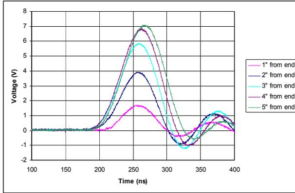
Figure 3: Buildup of helix voltage from transformer coupling with air dielectric.
