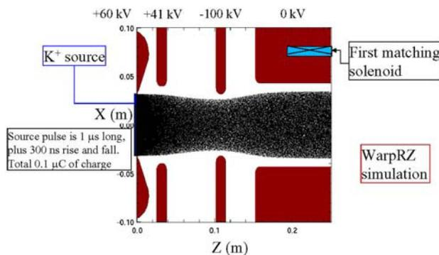
Figure 3: The Accel-Decel Injector.
