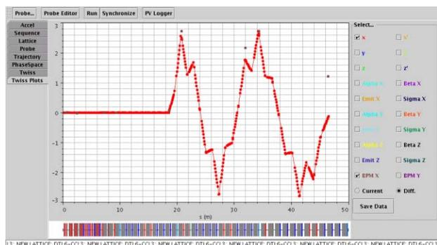
Figure 3: Orbit difference measurement after the dipole corrector magnetic field strength corrected.
