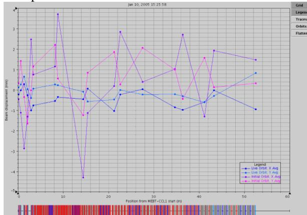
Figure 4: Orbit correction from the MEBT through CCL1. The four trajectories shown here are initial horizontal and vertical trajectories (purple and pink, respectively), and horizontal and vertical trajectories after correction (blue and light blue, respectively). The initial trajectory excursion is about 4 mm horizontally and 2 mm vertically. After correction, trajectory oscillation in both planes is within 1 mm.
