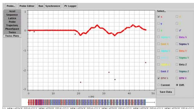
Figure 2: First orbit (trajectory) difference measurement for SNS DTL6 through CCL3. The solid line is online model calculation based on measured lattice and the dot points are BPM measurement.
