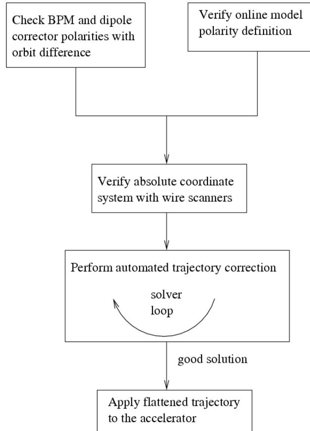
Figure 1: Schematic chart for trajectory correction procedures.
