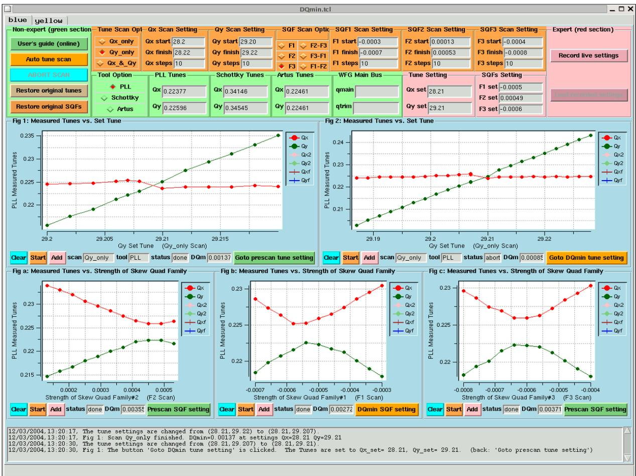
Figure 3: The graphical user interface of the “DQmin” application recorded in the RHIC e-log on December 3, 2004 during a coupling correction operation in the RHIC Blue ring. This operation successfully reduced the tune separation from 0.02 to 0.001.
