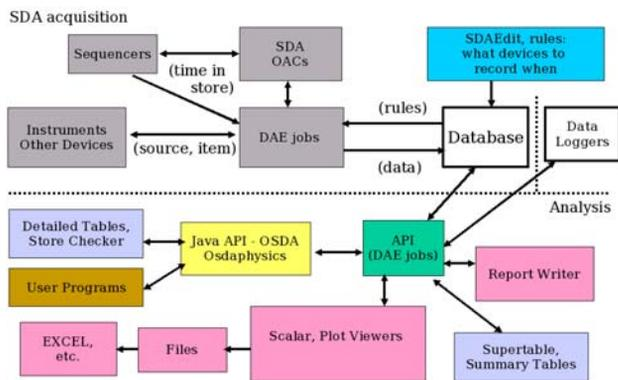
Figure 2: SDA data flow diagram.
