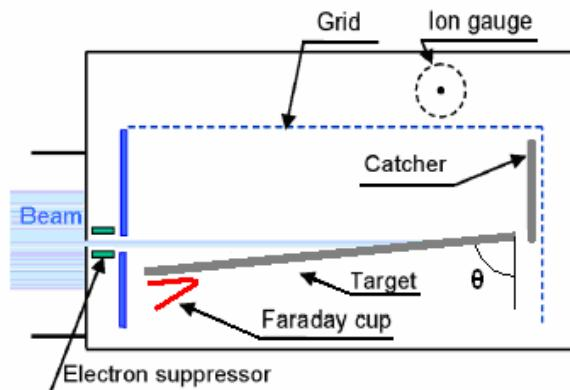
Figure 1: Gas-electron source diagnostic (GESD).
