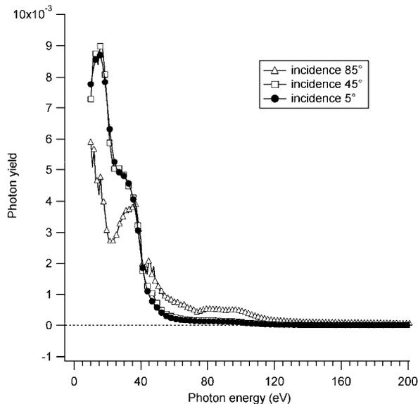
Figure 6: Photoelectron yield of the Al sample measured at incidence angles  $85^\circ, 45^\circ, 5^\circ$ .
