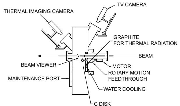
Figure 2: Schematic drawing of rotating carbon disk stripper.
