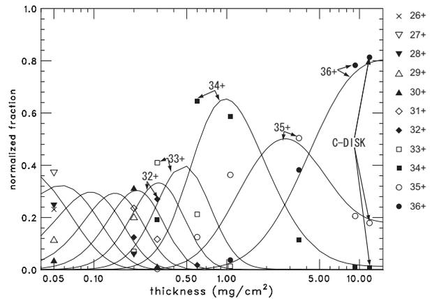
Figure 4: Charge state fractions of  $^{86}\text{Kr}$  at 46 MeV/nucleon. Axes are the same as Fig. 3. The charge state fractions are normalized by the sum of the measured charge state fractions. Solid lines indicate the calculations by GLOBAL.
