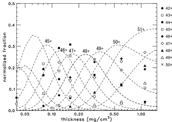
Figure 3: Charge state fractions of  $^{136}\text{Xe}$  at 11 MeV/nucleon. Horizontal and vertical axes indicate the thickness of the strippers and the charge-state fractions, respectively. The charge-state fractions are normalized by the area of the Gaussian fitted to the measured charge state distribution. Dashed lines indicate the calculations by ETACHA [12].
