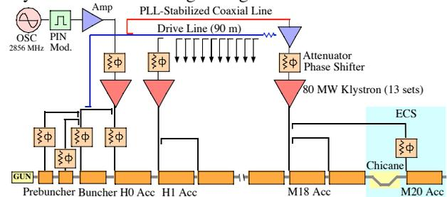
Figure 1: RF system of SPring-8 linac.
