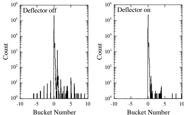
Figure 4: Satellite distributions of stored single bunch beam. RF powers for injector section were attenuated to be as low as possible to minimize the field emission for this measurement.
