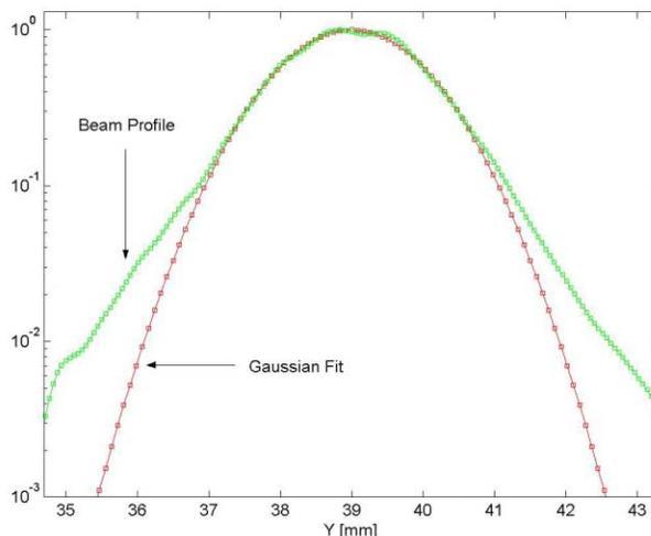
Figure 1: Plot of beam profile obtained from wire-scanner measurement. Over-layed is the profile of Gaussian fit.
