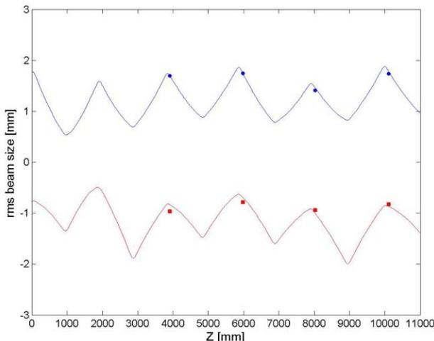
Figure 2: Plots of beam profiles. Solid lines are plots of beam size  $\sigma$  [mm] from the Trace3D program and dots are wire-scanner measurement data.
