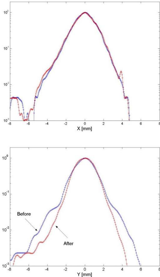
Figure 3: Plots of beam profile in X (top plot) and Y plane (bottom plot) from the wire-scanner in CCL module 1.
