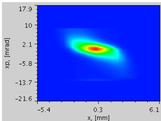
Figure 2: Horizontal emittance measurement in the MEBT at 38 mA peak current. The distribution has an rms normalized emittance of 0.29  $\pi$  mm mrad.
