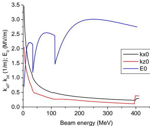
Figure 3: Wave numbers of betatron ( $k_{x0}$ ) and synchrotron ( $k_{z0}$ ) oscillations, real-estate accelerating gradient ( $E_0$ ) along the front end.
