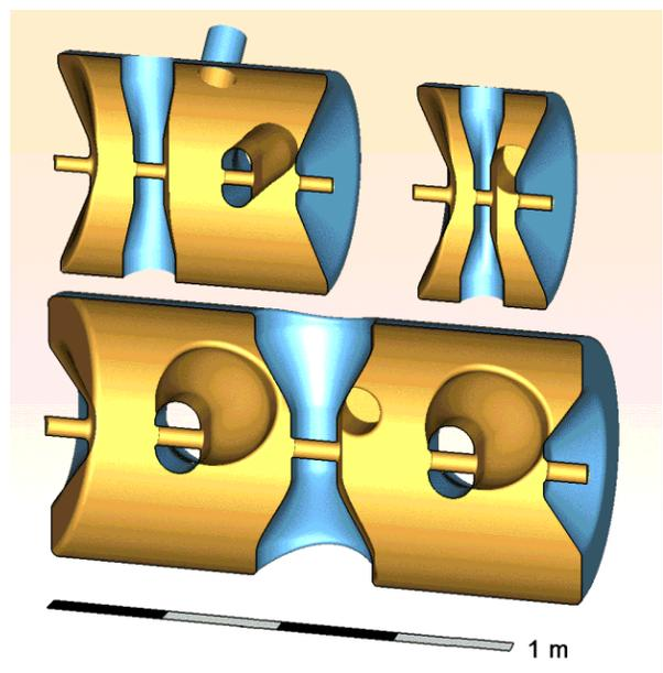
Figure 2: Cut-away view of the spoke cavities.
