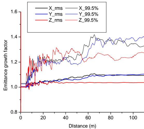
Figure 5: Emittance growth factor of the 28 mA beam along the front end.
