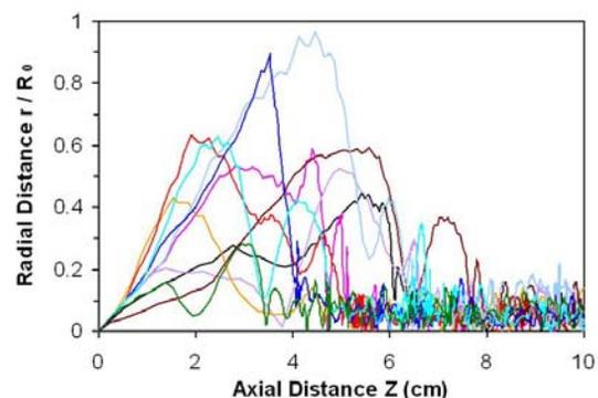
Figure 1: Monte Carlo simulation of trajectories of  $\text{F}^-$  ions in a RF quadrupole filled with 1.3 Pa He buffer gas. The ions have initial energy of 40 eV and enter the RFQ at an angle of 10 degrees.
