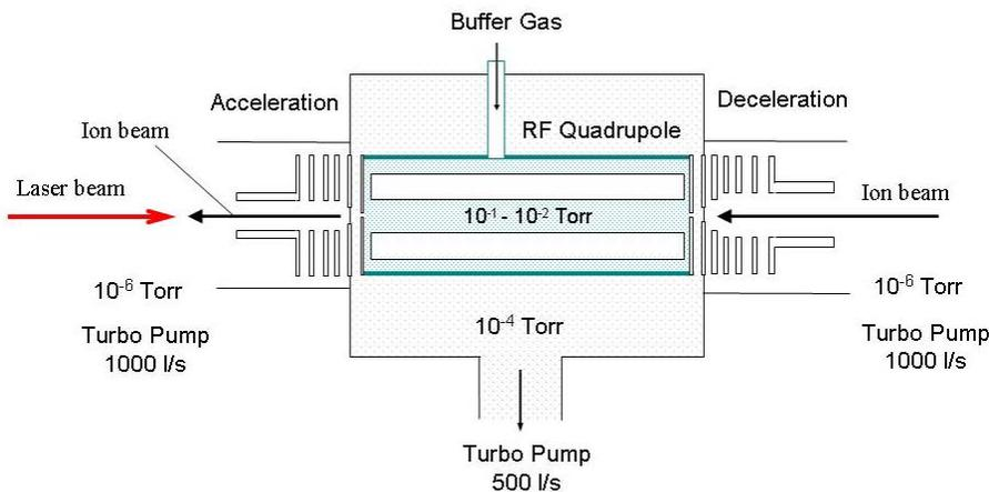
Figure 3: Schematic view of the gas-filled RF quadrupole ion guide.
