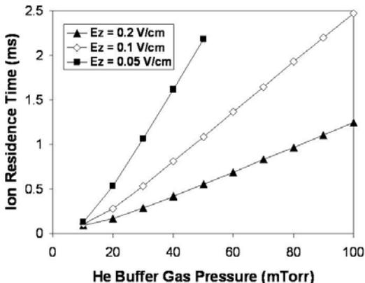
Figure 2: Calculated residence time of  $\text{Co}^-$  ions in a 40 cm long RFQ ion guide. The operation parameters of the RFQ are  $f = 2.76$  MHz,  $V_{rf} = 160$  V.
