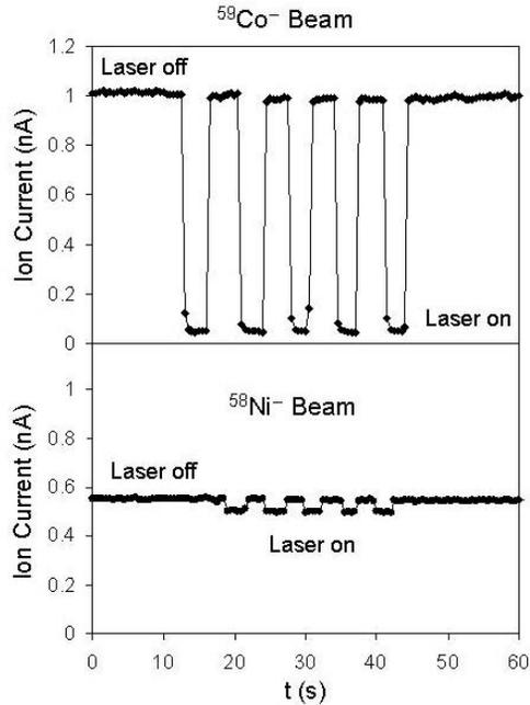
Figure 4: Measured intensities of ion beams accelerated from the RFQ with He pressure ~6 Pa. When the laser beam is turned on, 95% of  $^{59}\text{Co}^-$  and 10 % of  $^{58}\text{Ni}^-$  ions are neutralized.
