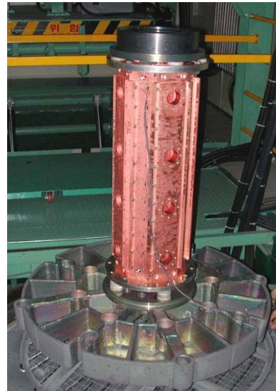
Figure 7: RFQ installed in furnace for brazing.
