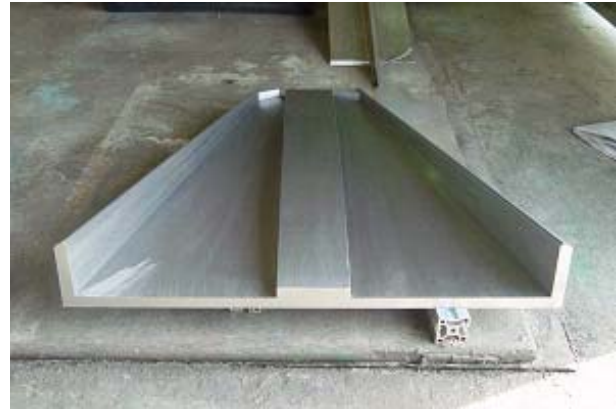
Figure 2: Power coupler under fabrication.
