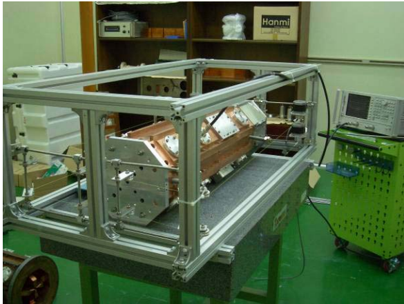
Figure 5: Field measurement setup for pre-brazing tuning.
