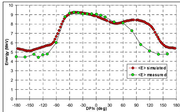
Figure 3: Average spectrum energy at RFQ exit as a function of phase difference between cavities.
