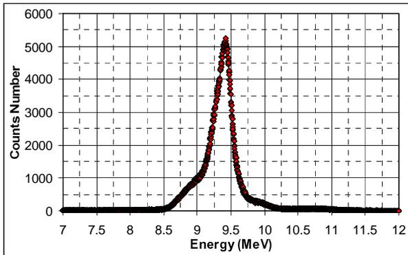
Figure 5: Energy spectrum out of the RFQ.
