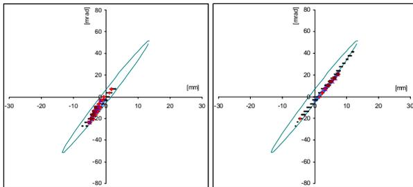
Figure 2:  $^{129}\text{Xe}^{17+}$  at LEBT end.  $E=4766$  KeV,  $\epsilon_x=0.0445$  mm-mrad,  $\alpha=-3.6$ ,  $\beta=0.87$  mm/mrad (left),  $E=4766$  KeV,  $\epsilon_y=0.0456$  mm-mrad,  $\alpha=-10.37$ ,  $\beta=2.88$  mm/mrad (right).
