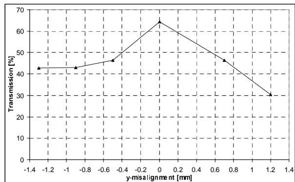
Figure 4: Beam transmission after vertical realignment of the LEBT.
