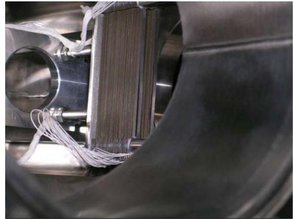
Figure 7: Beam profile monitor with a double grid reducing the effective step size to 0.5 mm.
