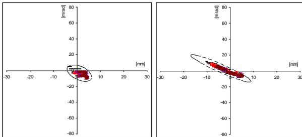
Figure 6: Horizontal and vertical emittance after the RFQ,  $^{16}\text{O}^{3+}$  Energy = 9400 KeV,  $\epsilon_{\text{rms},n,x} = 0.1093$  mm-mrad  $\alpha = 0.557$   $\beta = 0.58$  mm/mrad and  $\epsilon_{\text{rms},n,y} = 0.1205$  mm-mrad  $\alpha = 2.916$   $\beta = 2.309$  mm/mrad.
