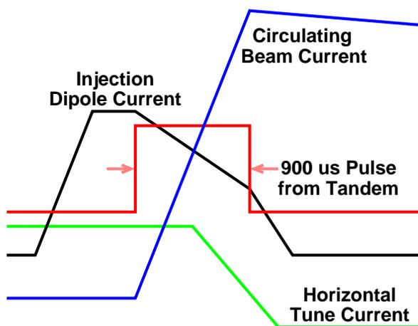
Figure 2: Typical timing at Booster injection.
