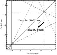
Figure 1: The tune spread of the injected beam on diagram. The energy width of the injected beam causes tune spread depending on the horizontal natural chromaticity.
