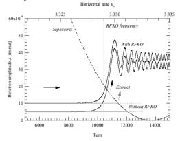
Figure 2: The schematic draw of extraction with phase space manipulation. The difference of betatron amplitudes when the electrons reached separatrix with RFKO decreases in the particular condition by comparison to the case without RFKO.
