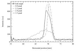
Figure 5: The measured distribution of the density of the extracted electron for various RF kick angles.
