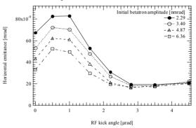
Figure 6: The extracted beam emittance estimated by tracking simulation for various RF kick angles and initial betatron amplitudes.
