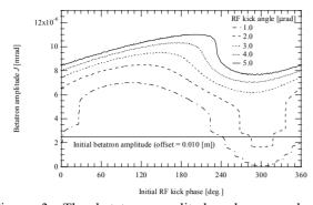
Figure 3: The betatron amplitude when an electron reaches separatrix. The emittance of extracted beam is affected by the kick angle and the initial phase of RF kick.
