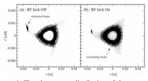
Figure 4: The phase space distribution of the extracted beam and the circulating beam before resonating at the location of the wire septum by the tracking simulation: without RFKO (a), with RFKO (b).
