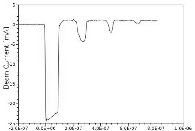
Figure 3: Results of the first multi-turn attempt on UMER (date: 5May'05). Beam current as a function of time measured at the first ring chamber.
