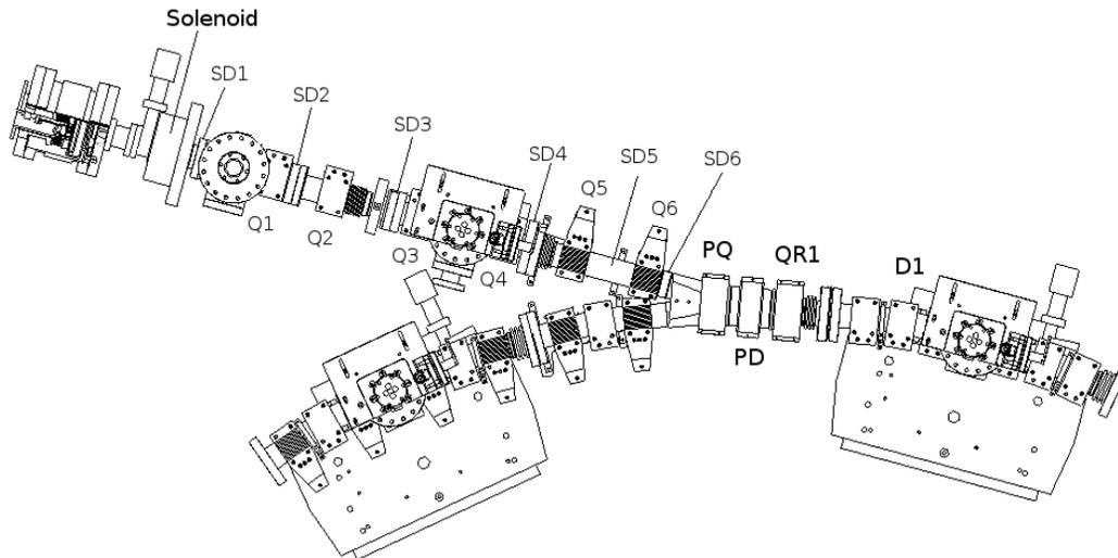
Figure 1: UMER injection line with quadrupoles Q1-Q6 and steering magnet SD1-SD6 positions labelled.
