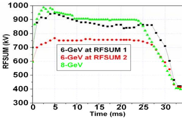
Figure 1(a) RFSUM 1 and RFSUM 2 for the 6-GeV acceleration and RFSUM for the 8-GeV acceleration are shown as the black, red, and green curves respectively.
