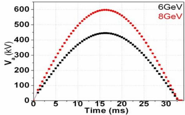
Figure 2(a) the accelerating voltages required by  $dB/dt$  for the 6-GeV and 8-GeV accelerations are shown as the black and red curves respectively.
