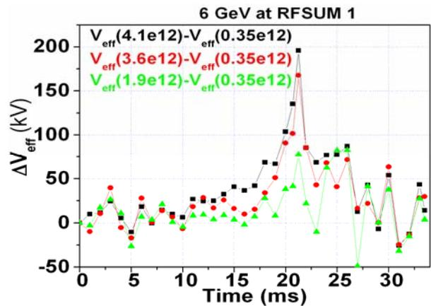
Figure 2(b) the  $\Delta V_{eff}$  between  $I_1$  and  $I_0$ ,  $I_2$  and  $I_0$ , and  $I_3$  and  $I_0$  are shown as the black, red, and green curves respectively.
