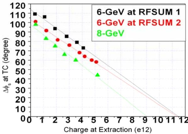
Figure 1(b)  $\Delta\phi_s$  vs. the extracted beam intensity at RFSUM 1 and RFSUM 2 for the 6-GeV acceleration, and RFSUM for the 8-GeV acceleration are shown as the black, red, and green points respectively; and their linear-fit results are shown as the black, red, and green lines.
