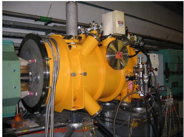
Figure 4: The cold snake installed in the AGS ring. Beam is going from left to the right in this picture.
