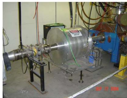
Figure 1: A barrier rf cavity in the Main Injector tunnel.
