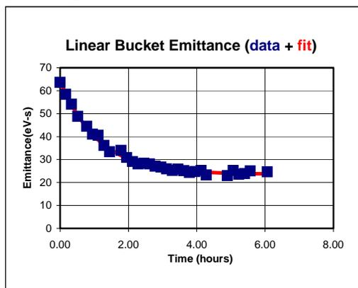
Figure 2: Linear bucket cooling: measured emittances and model fit.
