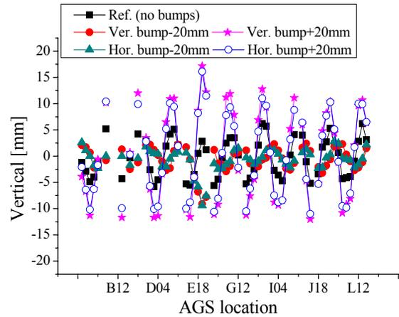
Figure 6: Vertical orbit in the AGS with horizontal and vertical bumping.
