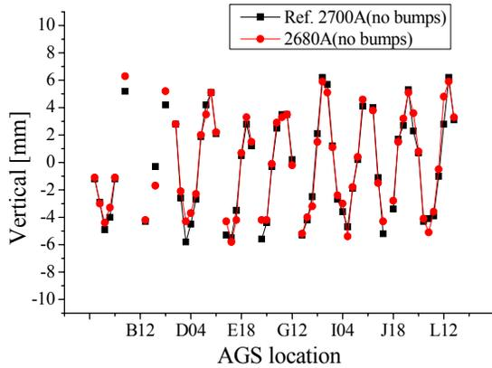
Figure 8: Current dependence of the vertical orbit.
