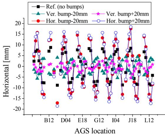
Figure 5: Horizontal orbit in the AGS with horizontal and vertical bumping.
