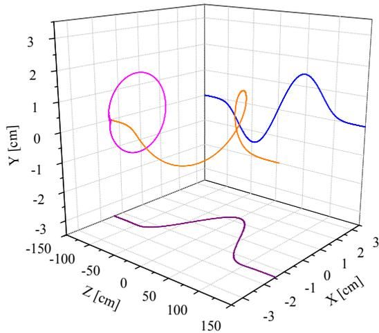
Figure 4: Trajectory of the 2GeV proton beam in the calculated magnetic field of the warm snake.
