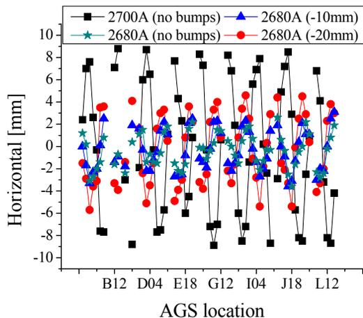
Figure 9: Horizontal beam orbit with 2680A and vertical bumping (Reference orbit is 2700A and no bumps).
