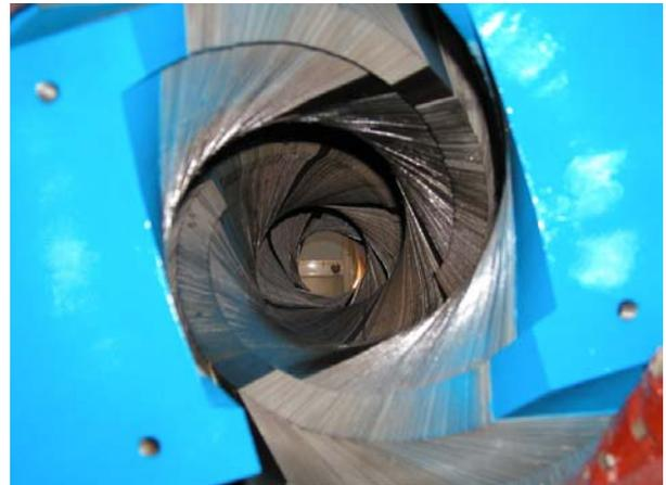
Figure 2: Helical dipole structure.
