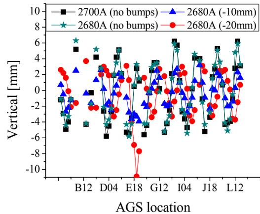
Figure 10: Vertical beam orbit with 2680A and vertical bumping (Reference orbit is 2700A and no bumps).
