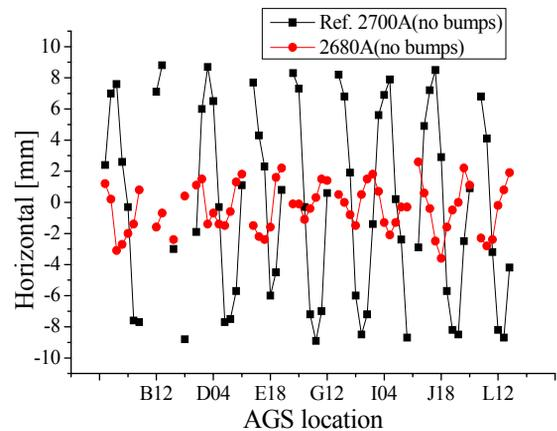
Figure 7: Current dependence of the horizontal orbit.
