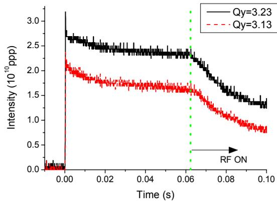
Figure 7: Comparing the beam-intensity when vertical tune is 3.23 with one when the vertical tune is 3.13.
