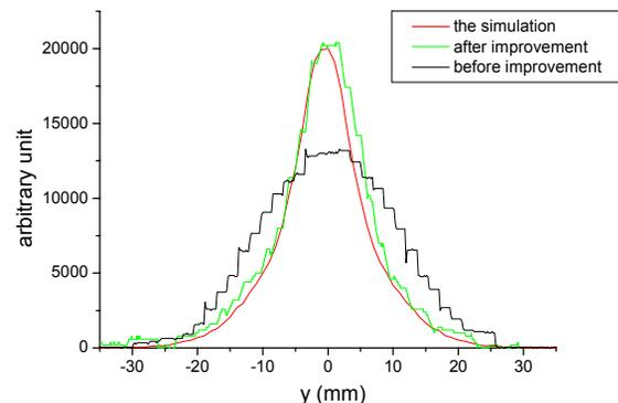
Figure 2: The vertical profile of the circulating beam. Black line is before the optimization and green line shows the beam profile with the new optics. Red line is beam distribution with the new optics by simulation.
