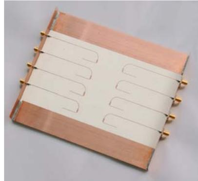
Figure 3: Test array of slot line pick-ups (rear side).
