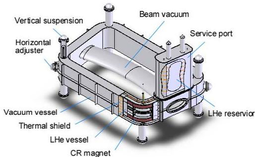
Figure 5: Cryostat structure of a CR dipole.
