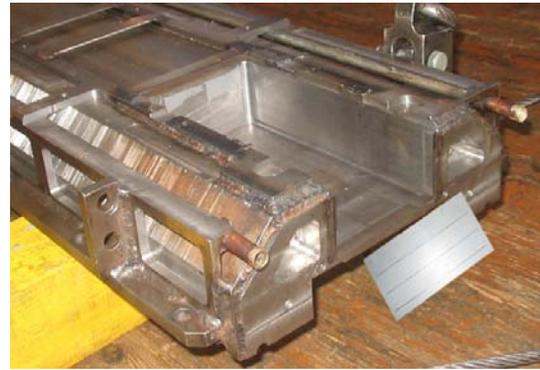
Figure 4: Preparation of the SIS100 test model PDP2 with improved yoke ends (laser-cut slits, reduced stainless steel end plate and minimized brackets).
