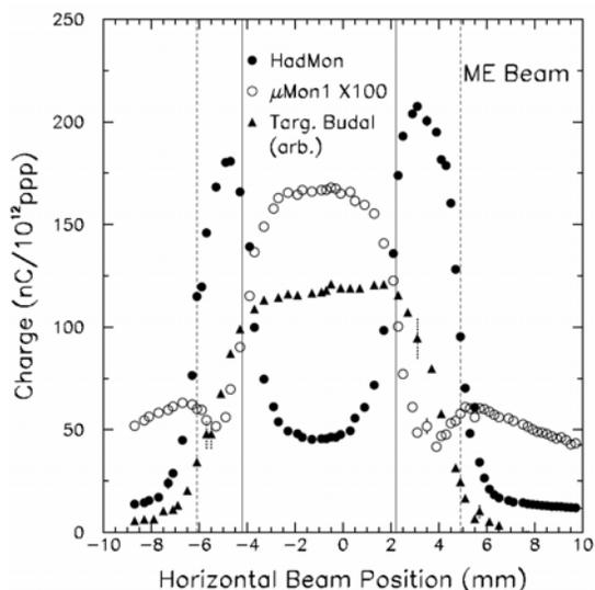
Figure 5: Signals from the Hadron Monitor, 1<sup>st</sup> Muon Monitor, and the target Budal monitor as the beam is scanned horizontally across the NuMI target. The solid (dashed) line represents the inferred outer (inner) edges of the target (collimating baffle).
