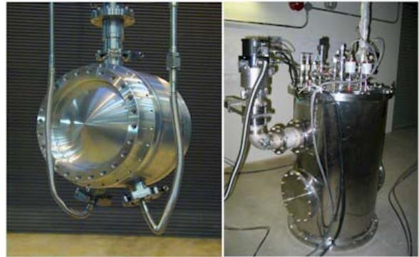
Figure 10: The KEK LH<sub>2</sub> absorber and its cryostat in the MTA at Fermilab.
