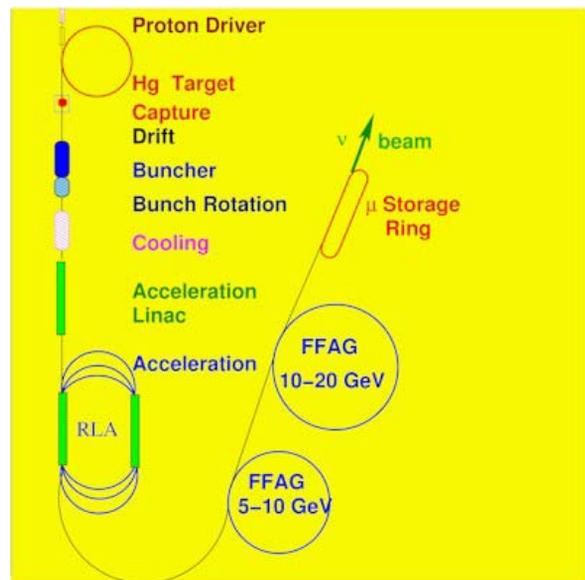
Figure 1: Layout of a generic neutrino factory studied by the MC.
