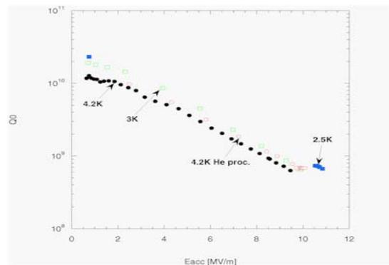
Figure 11:  $Q$  value deteriorates as the increase of accelerating gradients
