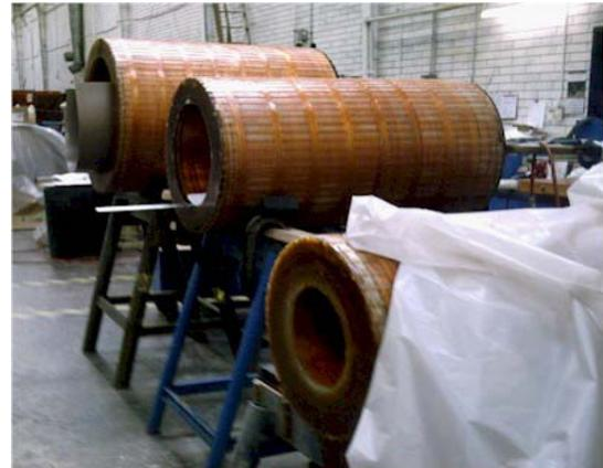
Figure 4: Targetry magnet coils during construction phase.
