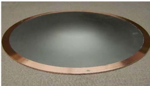
Figure 9: A 420 mm diameter and 0.38 mm thick curved beryllium window made by Brush Wellman Company.
