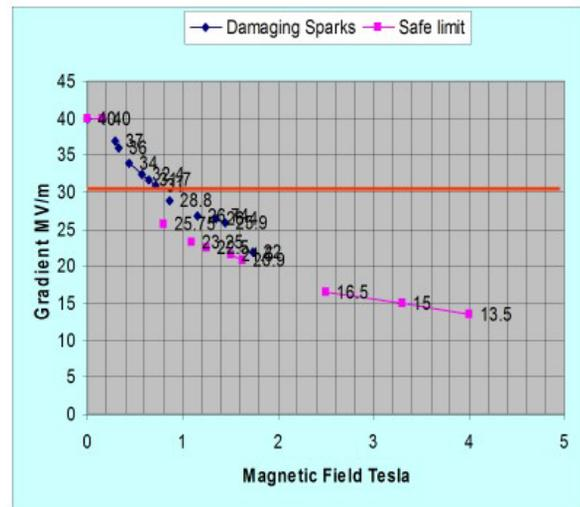
Figure 7: Experimental results of the achievable accelerating gradients for the 805-MHz pillbox cavity are plotted as a function of external magnetic field.
