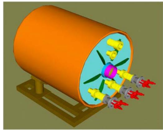
Figure 3: Design of the pulsed targetry magnet. The magnet has three nested coils that permit operation at 5, 10, and 15 T field. The magnet has a 15 cm warm bore and 1 m long beam pipe. The coils are normal conducting but cooled to liquid-nitrogen temperature to ease the requirements on the power supply.
