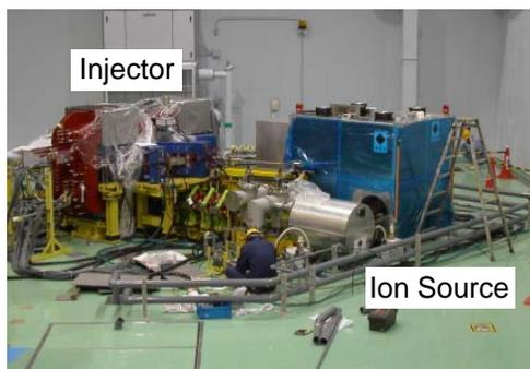
Figure 2: FFAG injector and ion source.
