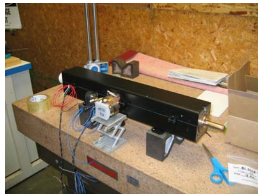
Figure 3: New 6 MeV accelerator section with shielding designed for less than 0.1% radiation leakage.
