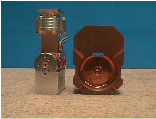
Figure 1: 1 MeV X-Band linear accelerator section (left) next to a single S-Band cavity.
