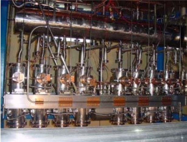
Figure 5: Eight resonators and a solenoid in first linac module ready to be loaded for a cold test.
