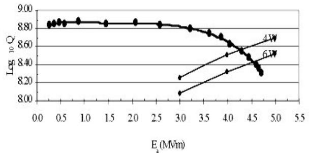
Figure 2: QWR-I1 cold test performance.
