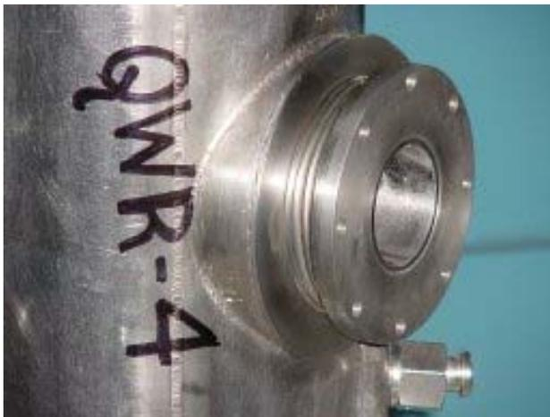
Figure 4: Coupling port bellow on a cavity after repair.
